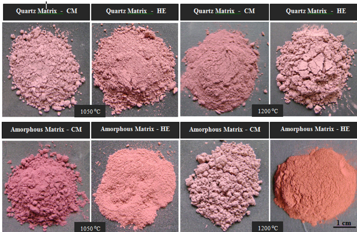
Fig. 6. Visual aspect of pigments (15 wt% of hematite) fired at 1050–1200 °C/2 h. CM, conventional milling; HE, high energy.
